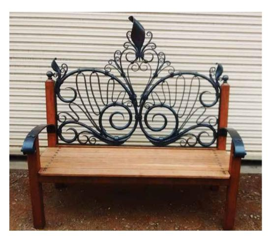
Garden seat forged mild steel and timber 1500 x 1350 x 600mm A back piece of free flowing scroll work inspired by traditional decorative design elements and techniques. Fitted into a neat fabricated steel and timber frame. Utilising steel sizes from 25mm to 12mm round, some flat bar; incorporating collars and rivets to accentuate the hand craftedness.
